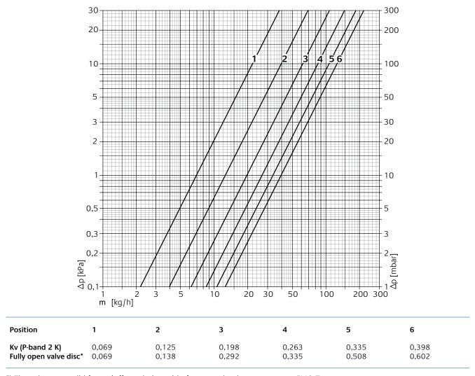
$<sup>^{*}</sup>$ ) The values are valid for on/off regulation with, for example, thermo actuator EMO T.
